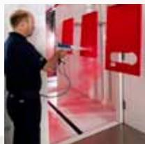
Unrestricted operator access around the product for manual touch up facilitates perfect results and simple, easy coating inspection.
