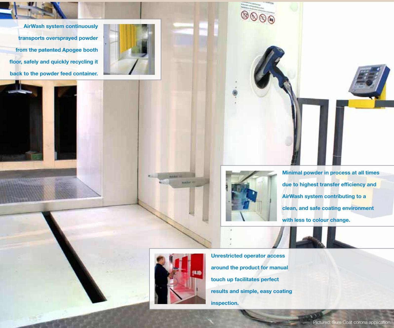
AirWash system continuously transports oversprayed powder from the patented Apogee booth floor, safely and quickly recycling it back to the powder feed container.
